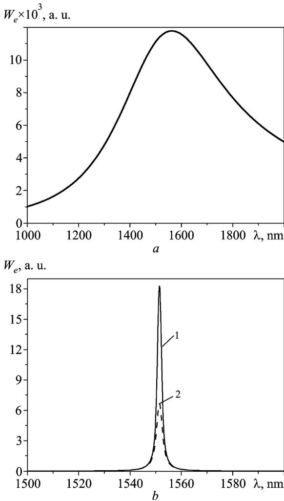
**Fig. 3.** Wavelength dependences of the luminescence intensity of a QD layer with thickness 210 nm placed on the silica membrane (a), and QD layer aggregated with metamaterials (b): 1 –  $\text{tg } \delta_a = 0$ ; 2 –  $\text{tg } \delta_{Si} = 10^{-3}$ . The units of graphs (a) and (b) have the same scaling
