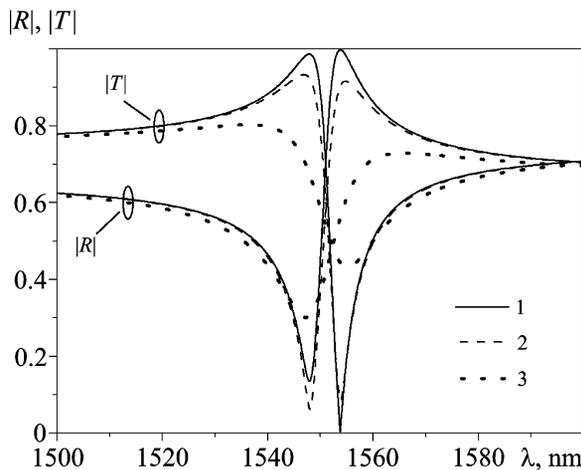
**Fig. 2.** Wavelength dependences of the reflection and transmission coefficients of the periodic array of silicon bars immersed in a non-pumped QD layer. Lines 1, 2, and 3 correspond to  $\text{tg } \delta_a = 0$ ,  $10^{-3}$  and  $10^{-2}$ , respectively
