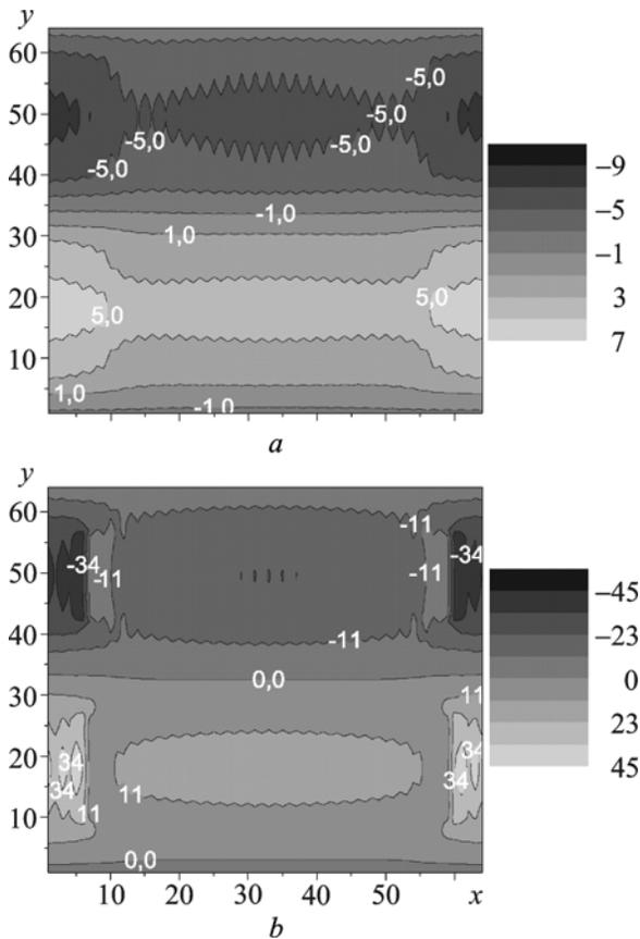
**Fig. 5.** Distribution of  $x$ -component of the electric field in the cross section of the array periodic cell ( $z = -50$  nm) for the nongained (a) and gained (b) QD layer aggregated with metamaterial at 1551.5 nm that corresponds to the maximum luminescence of the studied structure,  $\text{tg } \delta_{\text{Si}} = 10^{-3}$
