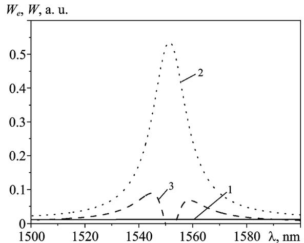
**Fig. 4.** Wavelength dependences of the photoluminescence intensity of a QD layer with thickness 210 nm (line 1), the energy absorption of the QD without optical pump aggregated with an array of dielectric bars,  $\text{tg } \delta_a = 10^{-2}$ , (line 2) and the photoluminescence intensity of metamaterials aggregated with QD (line 3)
