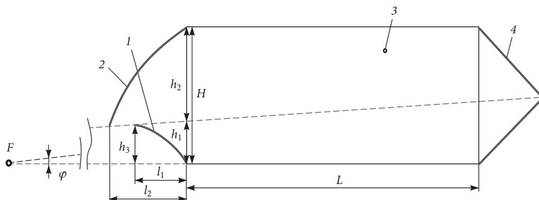
Fig. 7. Principal geometric parameters of the resonator
