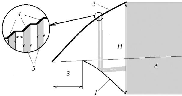
Fig. 6. Stepped surface of the concave cylindrical mirror
