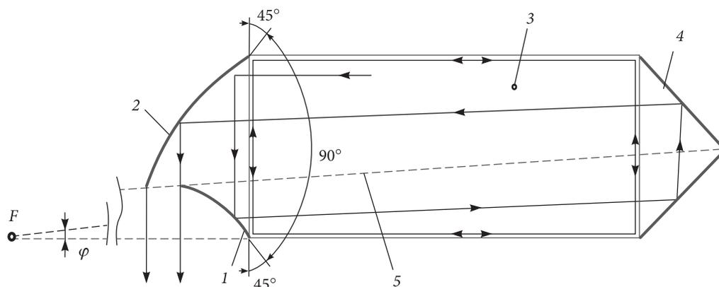
Fig. 4. Path of rays in a laser cavity with smooth expansion of the radiation beam cross section
