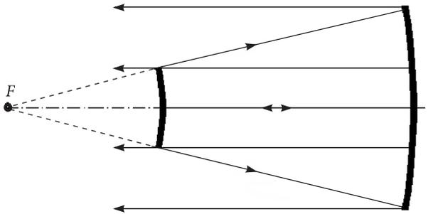
Fig. 2. Telescopic resonator
