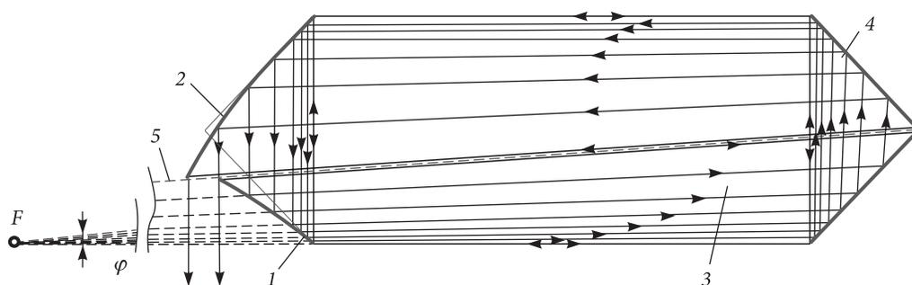
Fig. 5. Formation of a divergent laser beam in the resonator
