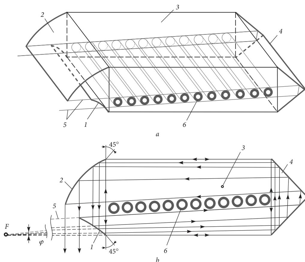
Fig. 8. Laser resonator with a smooth expansion of the radiation beam's cross section: pumping elements (a) inside the active material, and ray trajectories (b)
