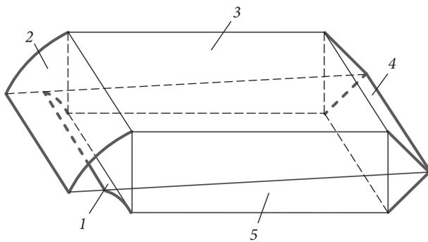
Fig. 3. Scheme of a laser cavity with a smooth expansion of the radiation beam cross section
