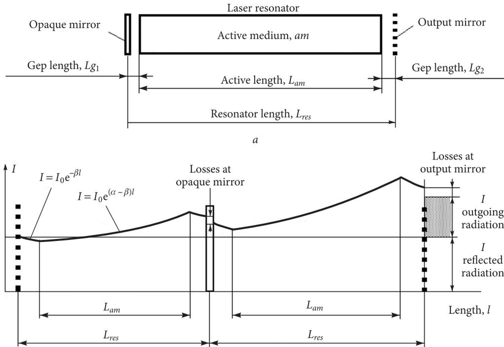
**Fig. 1.** Structural model of the laser resonator (a), and variations of the laser radiation intensity  $I$  in the direction  $l$  (b)
