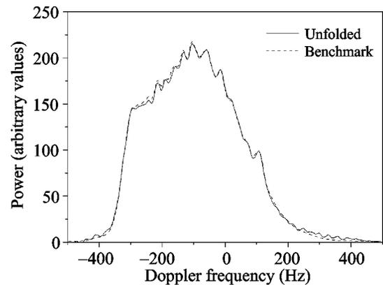
**Fig. 1.** Aliased spectra corresponding to PRF values of 500.0 and 529.4 Hz (decimation factors 18 and 17, respectively). The numbers of pulses per train are 170 and 180, respectively. Both spectra are results of averaging of 171 spectrograms
