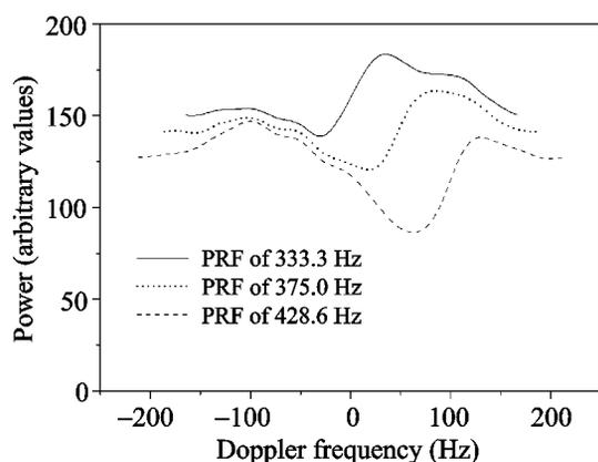
**Fig. 3.** Aliased spectra corresponding to PRF values of 333.3, 375.0, and 428.6 Hz (decimation factors 27, 24, and 21, respectively). The numbers of pulses per train are 168, 189, and 216, respectively. Each of the spectra is a result of averaging of 77 spectrograms
