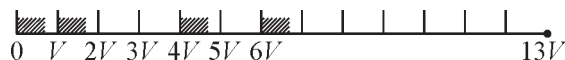
Fig. 2. The scheme of a four-section interferometer with one remote element. The element location areas are shaded. The added element is placed at the point d = 13V
