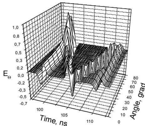
Fig. 3. Time and angle dependencies of amplitude of transversal electrical component for  $R = 30$  m
