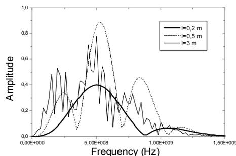
Fig. 4. Time dependence and frequency spectrum of amplitude of transversal electrical component for  $R = 30$  m and different  $l$
