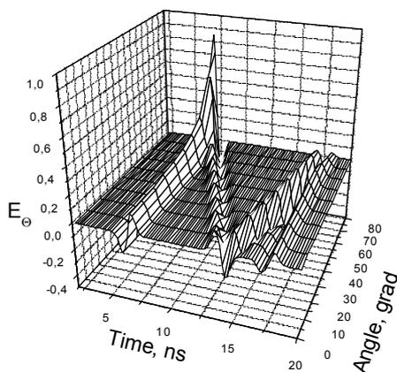
Fig. 2. Time and angle dependencies of amplitude of transversal electrical component for  $R = 2$  m
