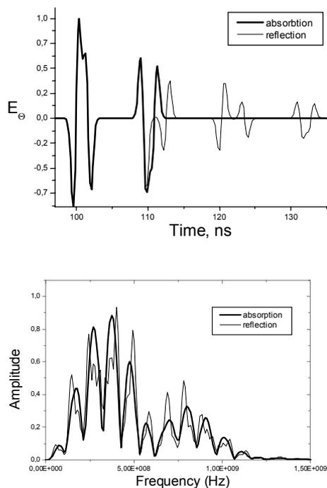
**Fig. 5.** Time dependence and frequency spectrum of amplitude of transversal electrical component for the cases of absorption and total reflection of current wave from source ( $R = 30$  m and  $l = 1,64$  m)
