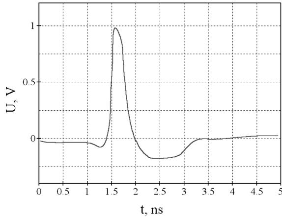
**Fig. 5.** The strobe pulse oscillogram with duration 0.25 ns, at the level  $0.5 U_{max}$
