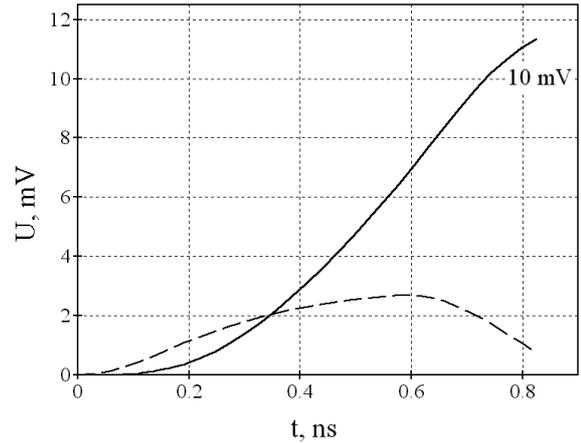
**Fig. 2.** The converted voltage step with the amplitude 10 mV; the dashed line shows a signal part passed through the diode capacitance
