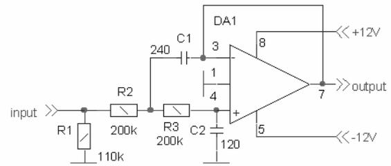
**Fig. 7.** The afterfilter circuit
