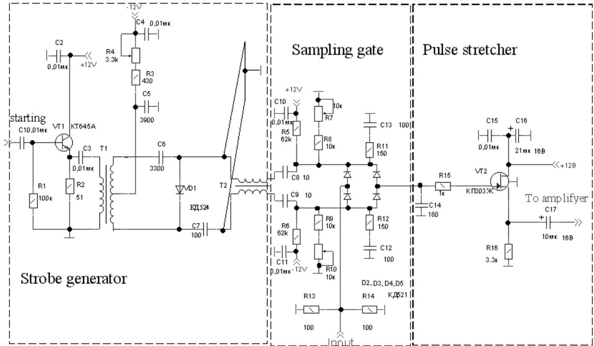
Fig. 1. The sampler circuit
