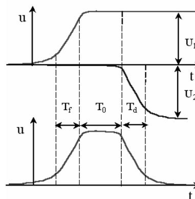
**Fig. 4.** The strobe pulse forming in the short-circuited line
