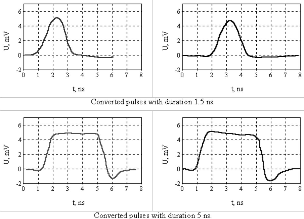
**Fig. 7.** Comparison of signal conversion by samplers of the oscilloscope C1-70 (left column) and georadar (right column)
