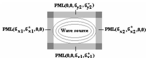
**Fig. 2.** Structure of a two-dimensional FD-TD grid having the Berenger PML ABC
