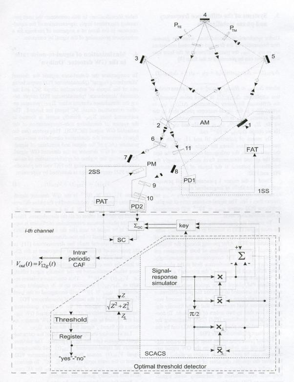
Fig. 1. Optical arrangement and block diagram of GW - detector "Dulkyn."
